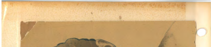
The glue turns brown, collects dirt, and can cause a color shift in photos.
