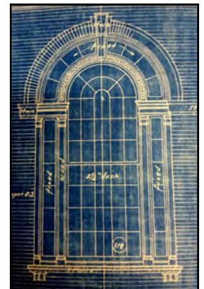
Blueprint drawing of the Palladian window used in the historic Post Office.
